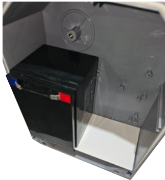
First battery placed in position
